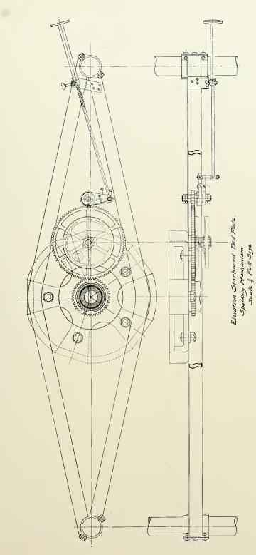
ENGINE OF AERODROME A. ELEVATION STARBOARD BED PLATE, SPARKING MECHANISM
